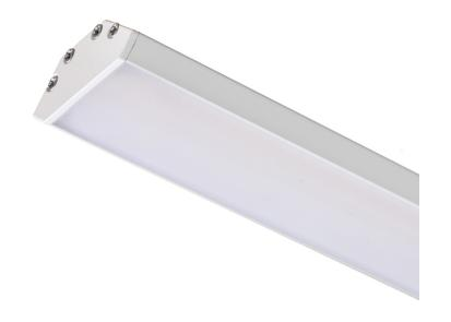
A corner aluminium profile for positioning suitable LED strips. Up to three 8-mm-wide LED strips or two 12-mm-wide LED strips can be placed in the profile. Supplied with a matt diffuser and accessories.
