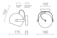
Round rotatable metal shade with a base, for use with a suitable E27 light source.
