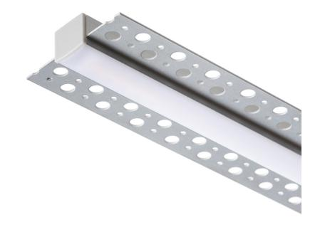
Aluminum profile for use with suitable LED-strip. Includes a matte diffusor and accessories. Suitable for recession into drywall.
