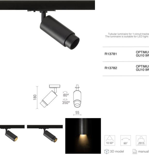
Tubular luminaire for 1-circuit tracks with the possibility of adjusting the light cone using a 10-50° zoom system. The luminaire is suitable for LED light sources with GU10 socket. Use light sources with a 120° beam angle in the luminaire to avoid unwanted shadows.
