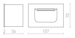
Recessed wall light with integrated LED. Suitable for indoor and outdoor use as orientation lighting of paths, stairs
