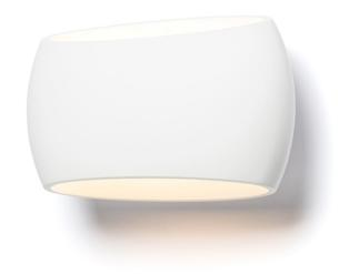
Rounded wall lamp of plaster for UP/DOWN illumination with an E27 socket and surface can be colored with interior paint.
