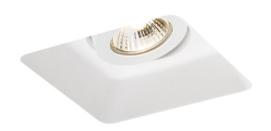
Recessed trimless downlight of plaster with a square opening. Surface can be colored with interior paint. Only for drywall installation.
