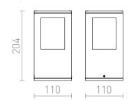
Outdoor die-cast aluminum light with shades of satin glass. Can be installed both as a wall light or bollard.
