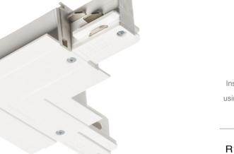
EUTRAC 3-circuit recessed track system made of extruded aluminium profile, which also serves as earthing. Inside, two embedded plastic profiles through which four copper conductors with a diameter of 2.5 mm are routed. Any profile can be easily cut to the desired length. The ends of the wires do not need to be cut or bent. When using halogen sources, the minimum installation height is 2.5 m. Below this height we recommend replacements in LED sources.
